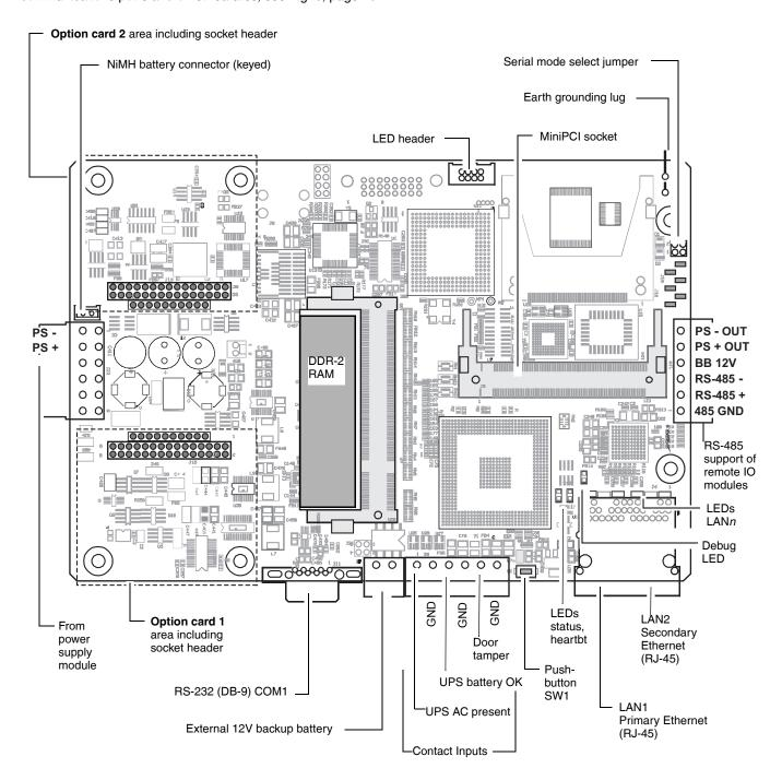
Fig. 5. WEB/CP-700 main board layout details
